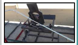
This system allows the Instructor to run training drills on moving steel targets that drop only when accurately hit. The target then returns to the upright position when the trolley turns around at the extreme of its travel. Multiple shooters on the line can sequentially engage the target efficiently.
