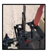
The innovative system incorporates a proprietary 12 VDC drive mechanism that resets the Threat target upright in 3 seconds.
