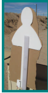
Hits to any part of this reactive target illuminate a red strobe.
