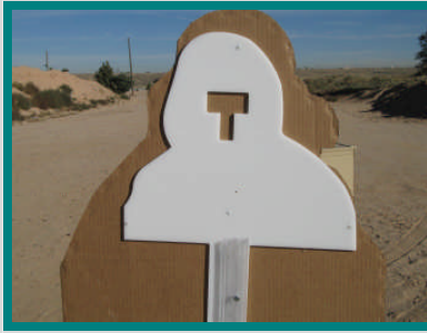
An inaccurate shot that hits any part of this reactive target illuminates a yellow strobe.
